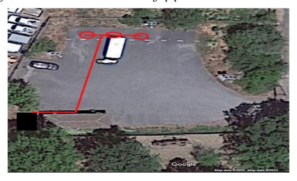
Figure 3: Current Plan for Installation of Charging Equipment Fort Bragg
