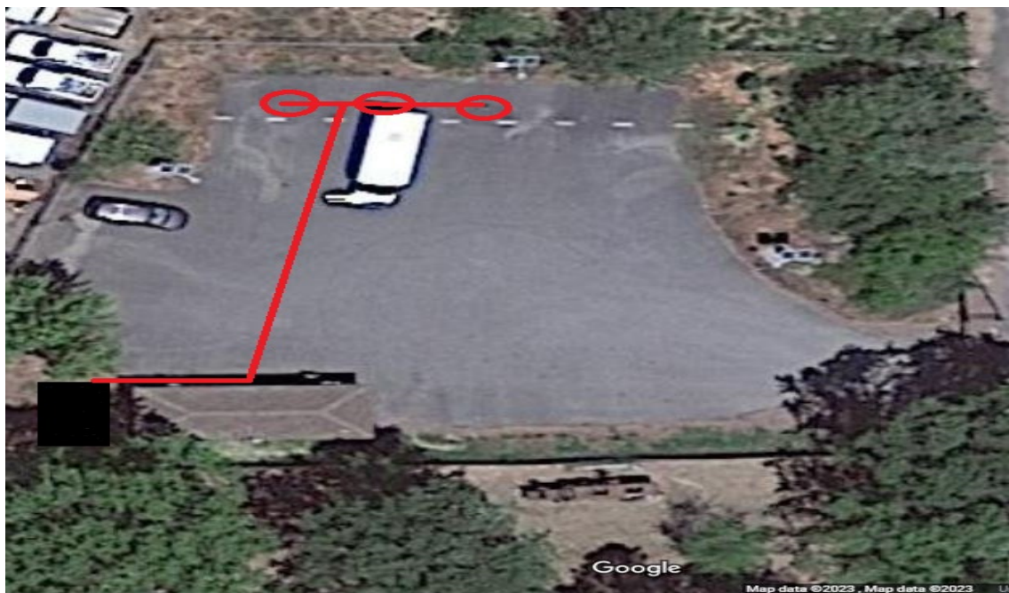
Figure 2: Current Plan for Installation of Charing Equipment Willits
