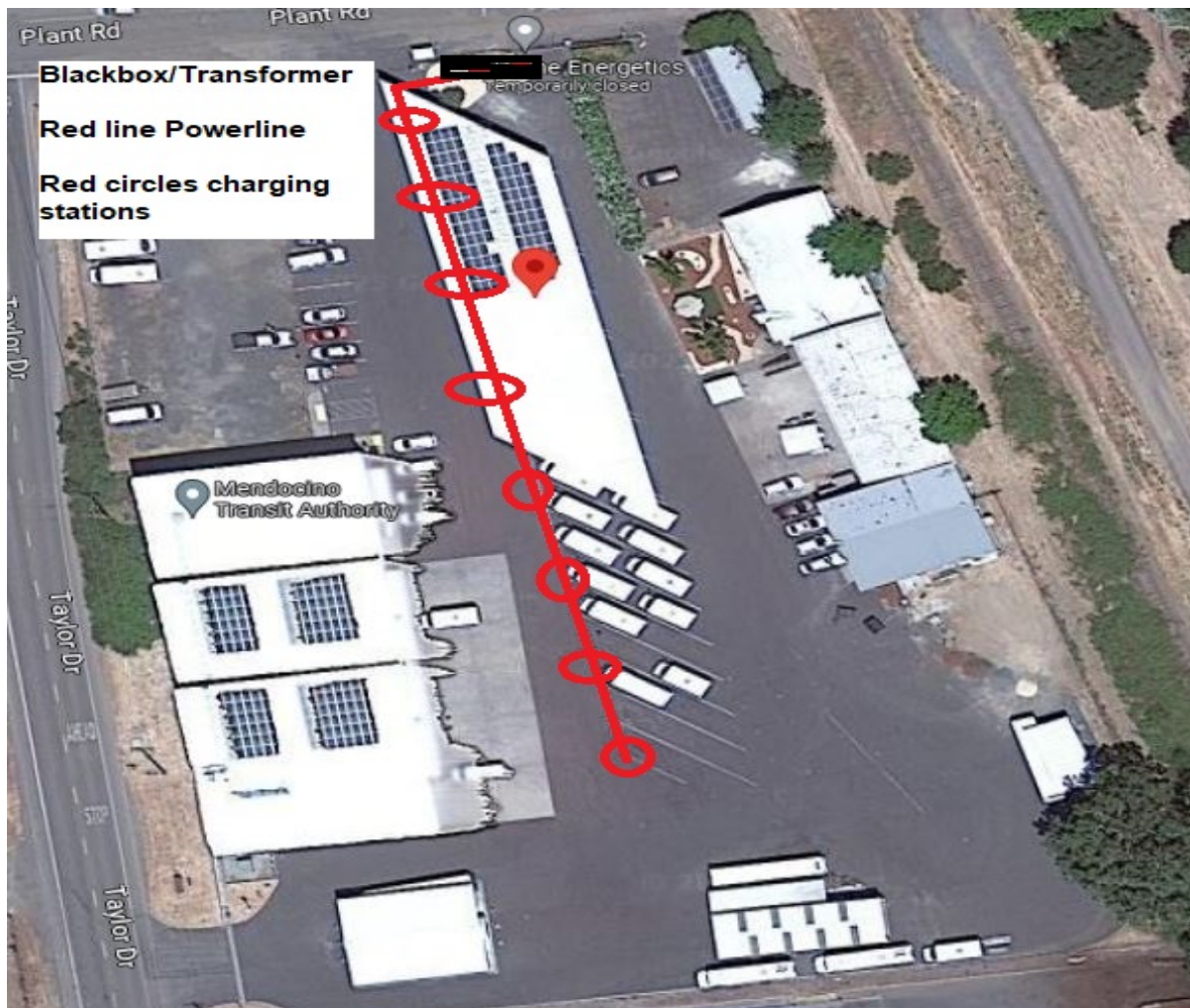
Figure 2: Current Plan for Installation of Charing Equipment Willits
